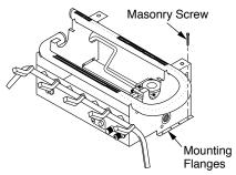
Figure 12 - Attaching Base Assembly to Fireplace Floor
